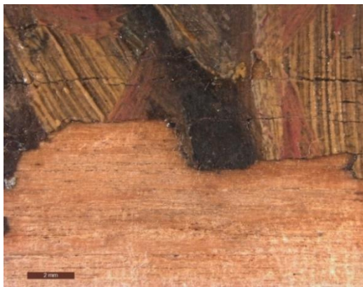
Figure 23. Micrograph. Raw plywood revealed by an area of paint loss.
