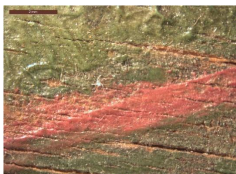
Figure 22. Micrograph. Periodic horizontal checking and associated paint loss.
