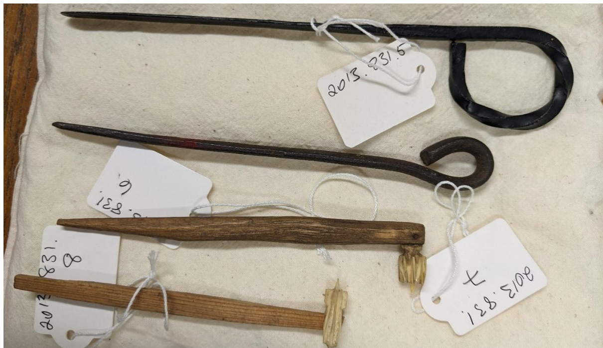
Figure 8. Straw-splitting 'engines', two iron and two wooden and bone, once used by Hannah Freeman.
