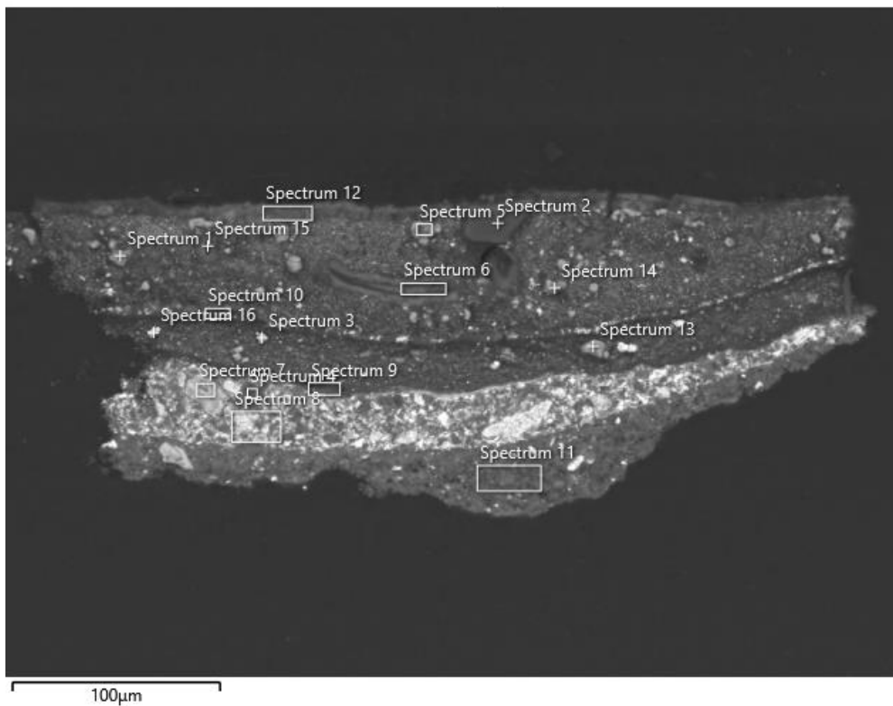
Figure 63. The Barred Gate , paint cross-section A, SEM-EDX image. The white sections indicate the areas analysed for EDX spectrum. Courtesy of The Department of Conservation, The Courtauld Institute of Art.
