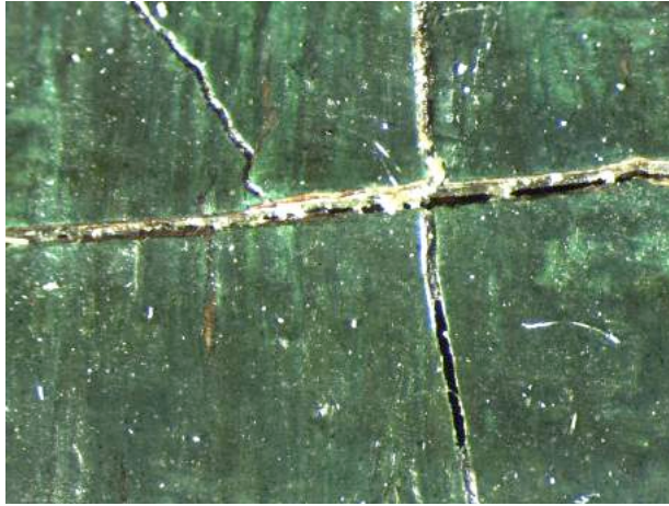
Fig 17. Photo-micrograph of drying crack showing bright orange/pink painting beneath The Church near Carrieres-Sur-Seine . (Photograph Cleo Nisse)
