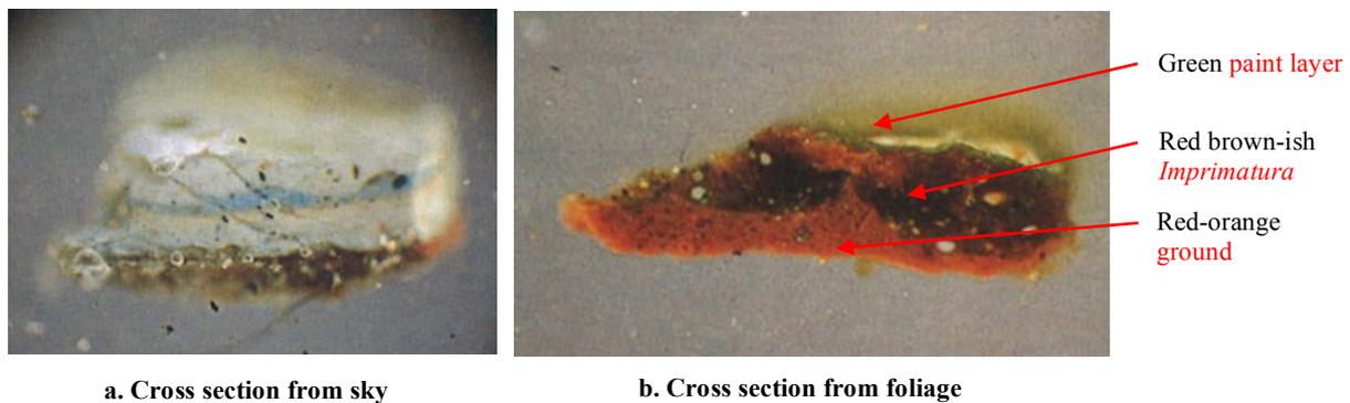
**Figure 18: Cross sections from Paolo Bensi's technical study of Magnasco's *Trattenimento*.**
