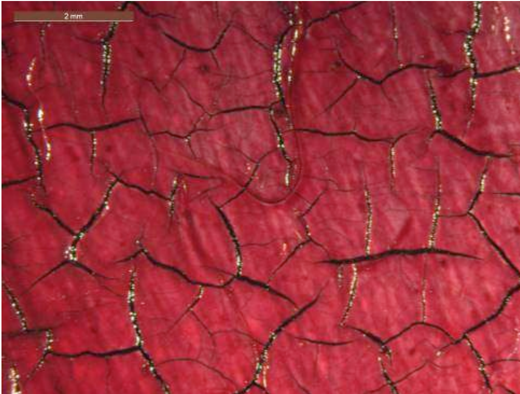
Fig. 38: Micrograph Showing an Area of Crimson Robe where each Red Lake Paint Layer Appears to Have Been Allowed to Dry before the Next is Added
