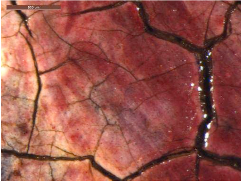
Fig. 44: Micrograph Showing Ultramarine Layer with Red Lake Layer Above, Creating the Purple-Pink of the Book Cover
